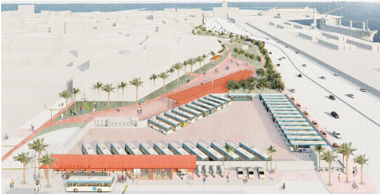
Figure 7 - North view of the Terminal with the proposal for the location of different types of vehicles, chargers and infrastructure intervention. (Source: Design studio of TUB).
