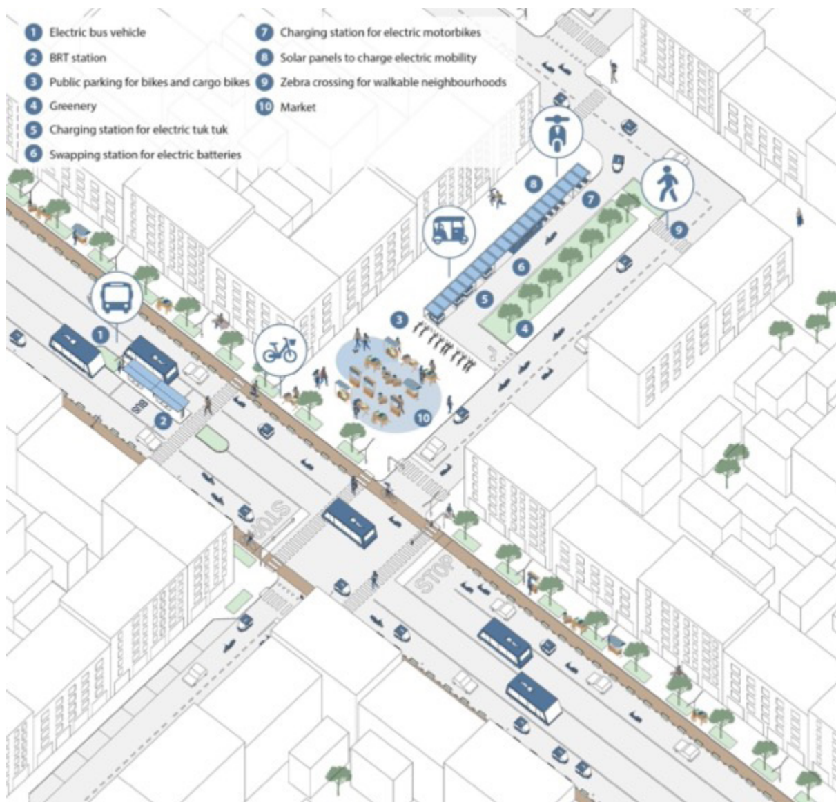
Fig. 12 Multimodal hub, Example 2 – Integration of electric Bus Rapid Transit (BRT) services, bicycles and e-bike parking, electric tuk-tuks and motorcycles with improved pedestrian infrastructure (UN-Habitat)
