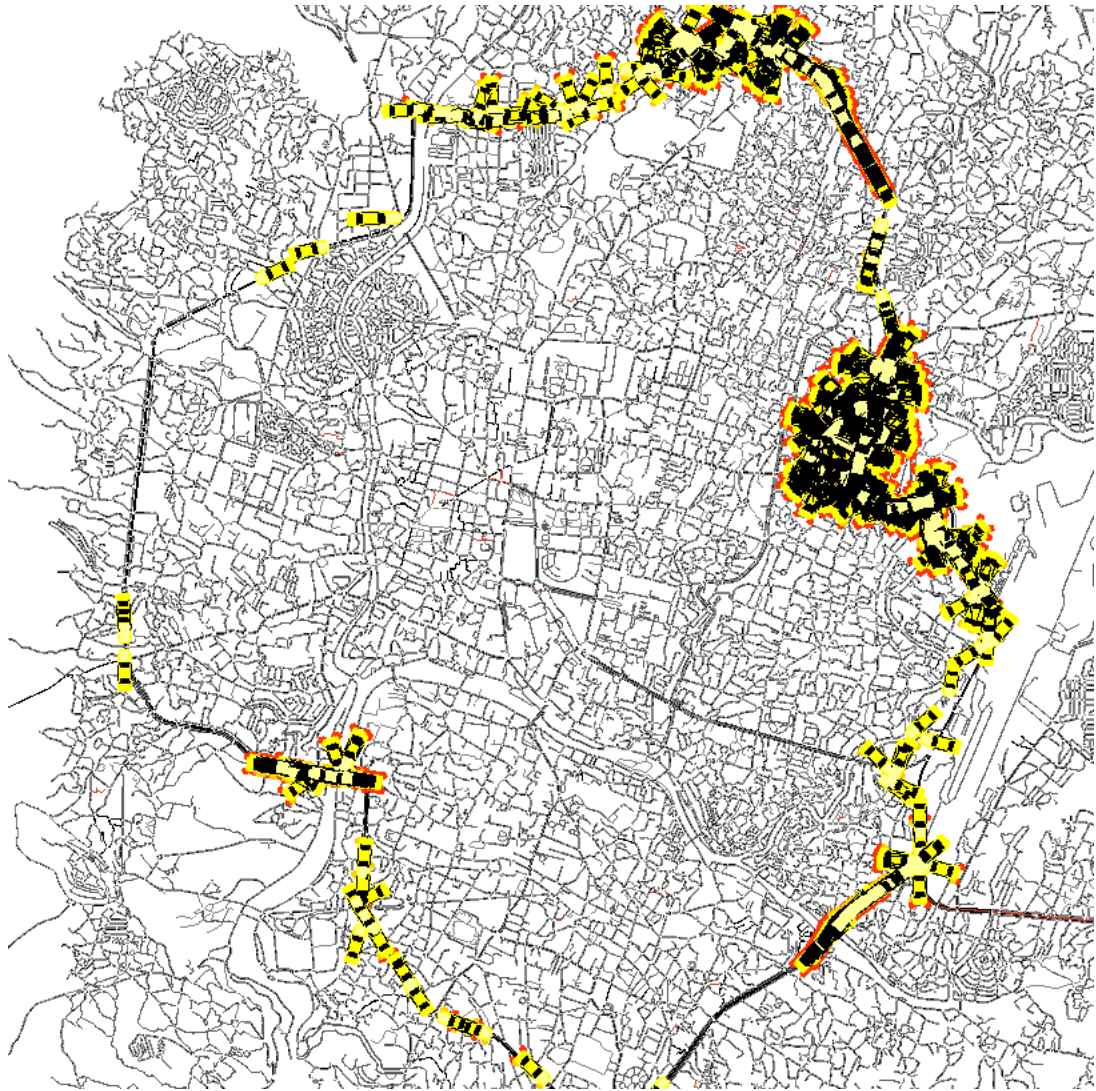
Fig 3.4. Simulated traffic congestion on ring road influenced by adjoining junctions and traffic mix leads to spatial-temporally confined high traffic emissions episodes
