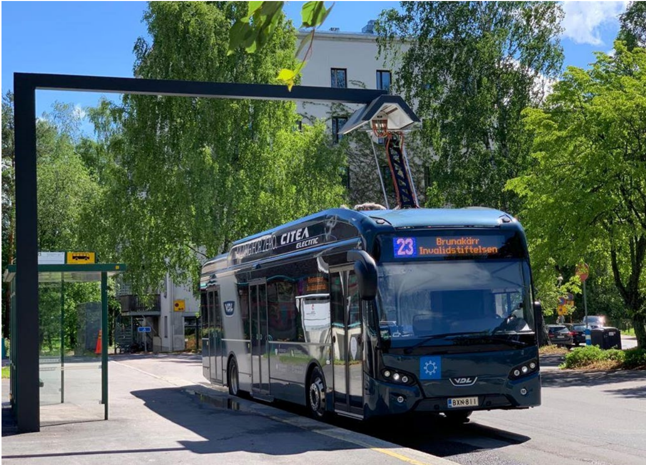
A VDL Citea SLF-120 Bus with pantograph charging in Helsinki, Finland (2019):
