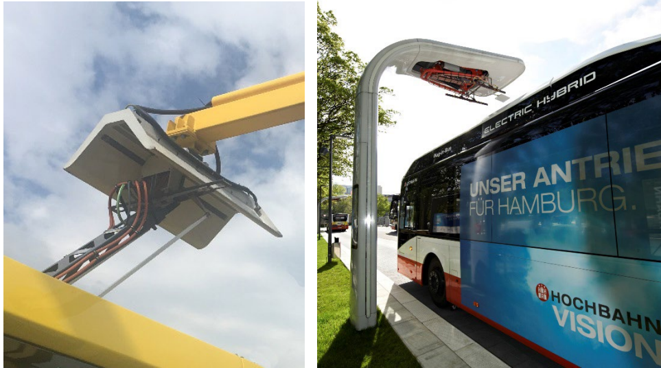
Fig. 7. Schunk Smart charging contact system and inverted pantograph
