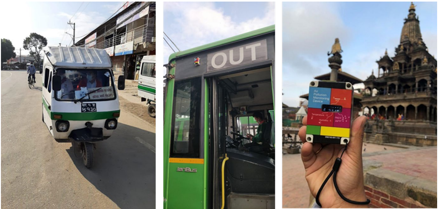
Figure 10. Modes of transport in Kathmandu. Left: Electrified Tempo minibus with open-seneca sensor mounted on the roof. Centre: open-seneca device mounted on the side of a Sajha Yatayat bus. Right: walking volunteer presenting the open-seneca sensor in front of a temple in Kathmandu.
