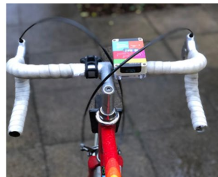
Figure 1. open-seneca air quality sensor, with main characteristics and mounting mechanism.
