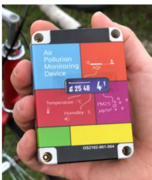
Figure 1. open-seneca air quality sensor, with main characteristics and mounting mechanism.
